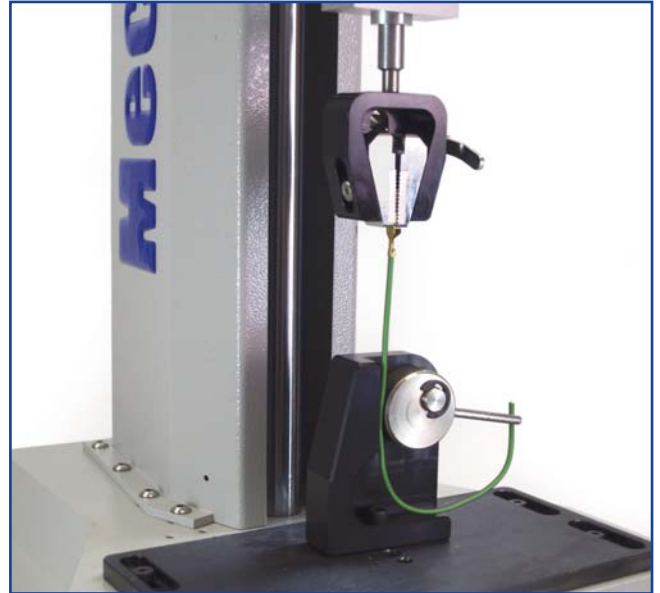
Cable Cam Grip shown with Wedge Grip testing crimp terminals
