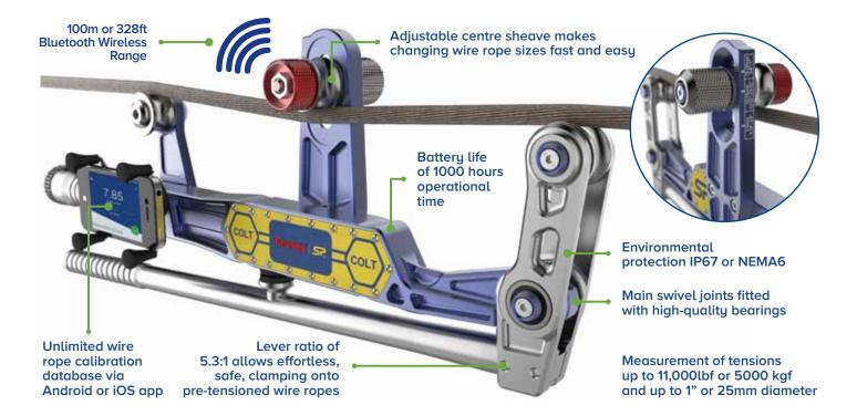
The Crosby Straightpoint COLT is a lightweight wire rope tension meter, for fast and accurate measurement of tensions up to 11,000lb or 5000 kg and up to 1" or 25mm diameter.
