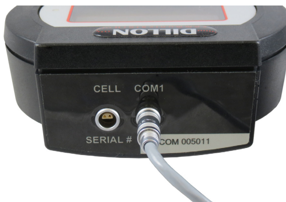
Figure 2.7 External Power Supply Connection (Communicator)
